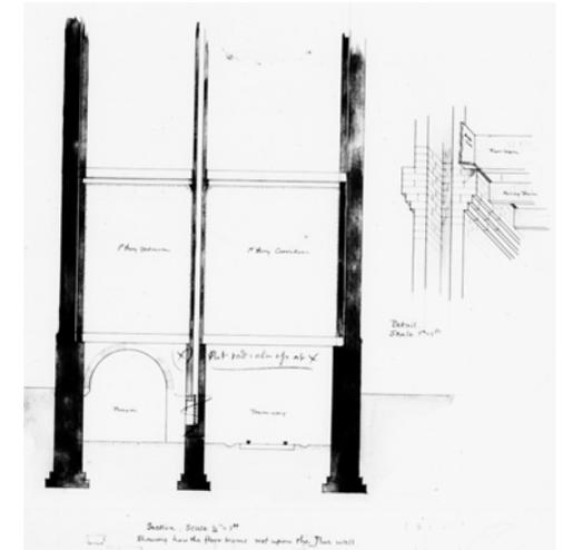
Fig.A.41 Section showing support of floor beams, Buffalo State Asylum
