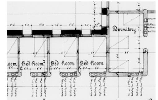
Fig A.19 Detail of a typical floor plan, Buffalo State Insane Asylum, showing shafts in the internal corridor wall for forced air circulation
